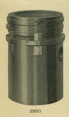
and unbolt the rod. Turn crank to out position. The piston may now be withdrawn. Clean with gasoline or a hot solution of lye and water. Loosen the rings and clean the grooves. Oil the piston well before replacing. In replacing piston turn it bottom side up so that the stop pins can be seen, otherwise the rings may be broken. Be sure to turn it right side up before connecting up rings can be removed from piston by taking three strips of tin about one-half inch wide and six inches long, slip
